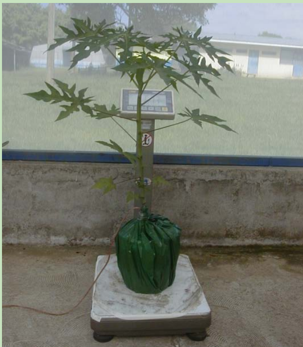
Figure 1. Experimental set-up for gravimetric verification of sap flow measurements performed by the HRM. Whole papaya plants growing in pots filled with potting mix were wrapped to prevent soil water evaporation (see Gutiérrez, Harrington, Meinzer and Fownes, 1994).
