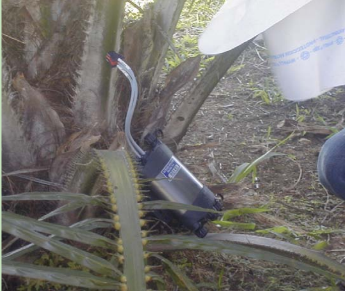
Figure 2. HRM probes installed at the base of a fully expanded leaf in a 1-year-old oil palm growing in the field in Coto 49, Palma Tica, South Pacific of Costa Rica. An oil palm leaf at this age may be 2,5 m long.
